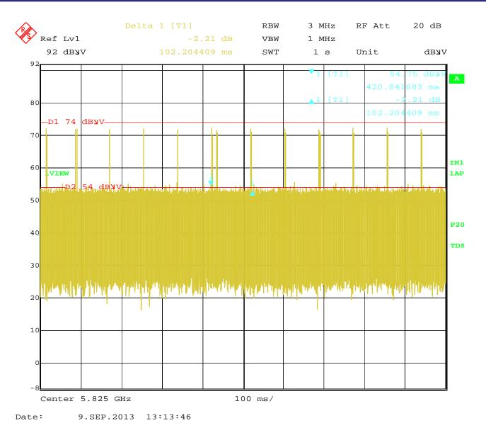
Actual Operation of the Roku when the Fast Forward button was hit continuously. -1 Second Scale Duty Cycle = (14\*601.202405 us) / 1000 ms = 0.8417%
