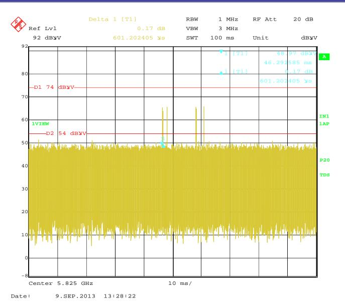
Actual Operation of the Roku when the Fast Forward button was hit continuously. – 100 mS Scale Duty Cycle = (4\*601.202405~uS) / 100~ms = 2.4045%
