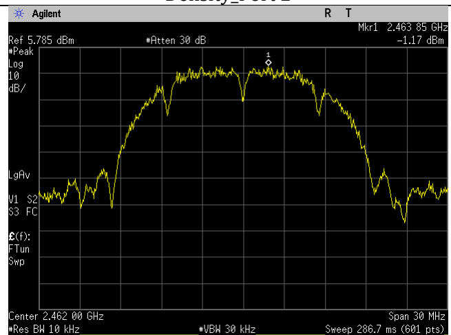
High Ch_2462MHz_20MHz BW_b-mode_Spectral Density_Port 2
