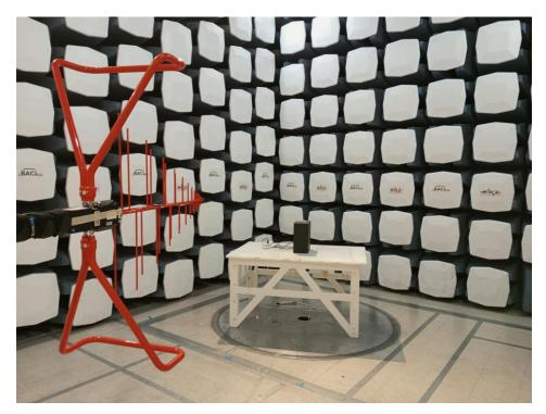
1.2 Radiated Spurious Emissions: 30 MHz – 1 GHz Rear View at 3 meters
