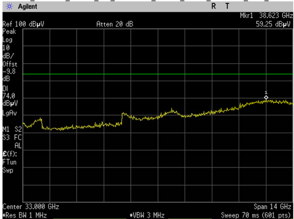
U-NII-3_5745MHz_Low Ch_149_20MHz BW_n-mode_15.209_26-40GHz_Peak_Port 2
