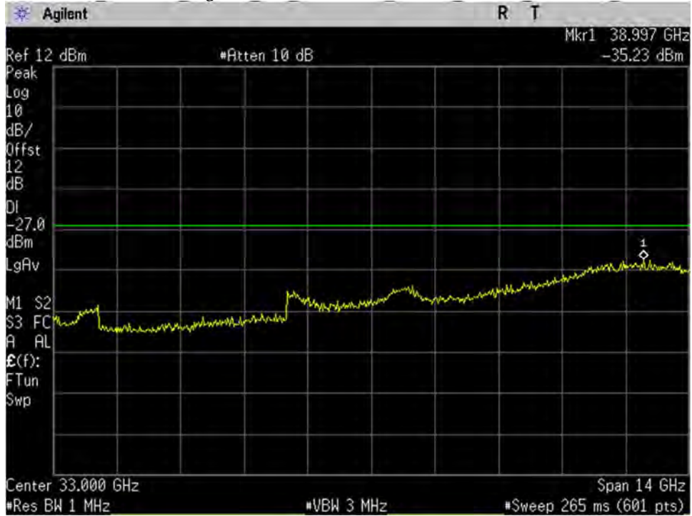
U-NII-2C_5710MHz_High Ch_142_40MHz BW_n-mode_-27dBm_26-40GHz_Port 1
