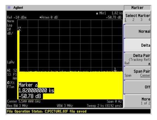
Note: the communication between EUT and router was set to 5530 MHz and 80 MHz channel bandwidth. However, 5500 MHz is the primary channel that contains the control signal. Therefore, it was monitored for the non-occupancy period.
