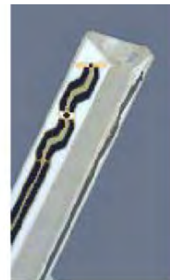
Figure 2.3 Probe Thick-Film Technique
