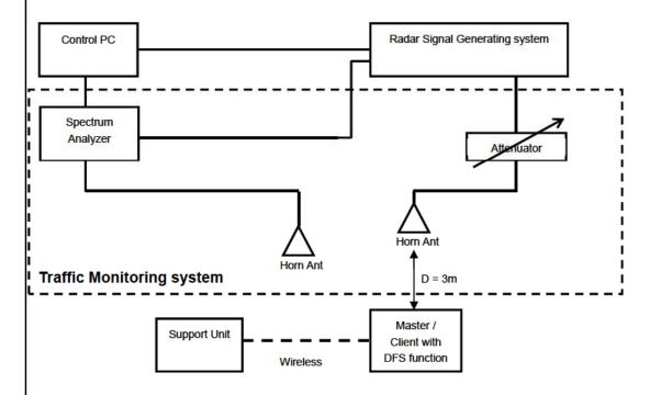
The UUT is a RLAN device operating in Client mode. Radar test signals are injected into the UUT.
