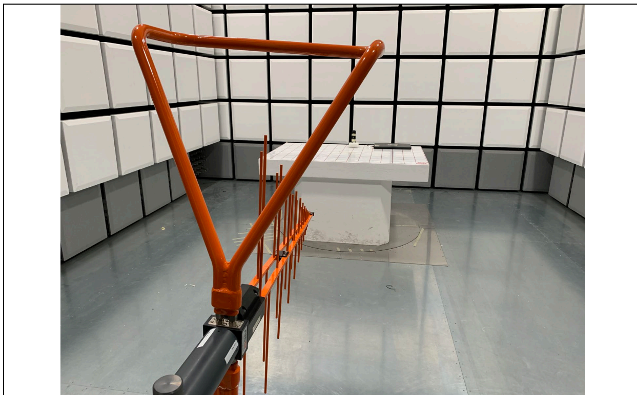
Radiated Emission Test below 1GHz Front View
