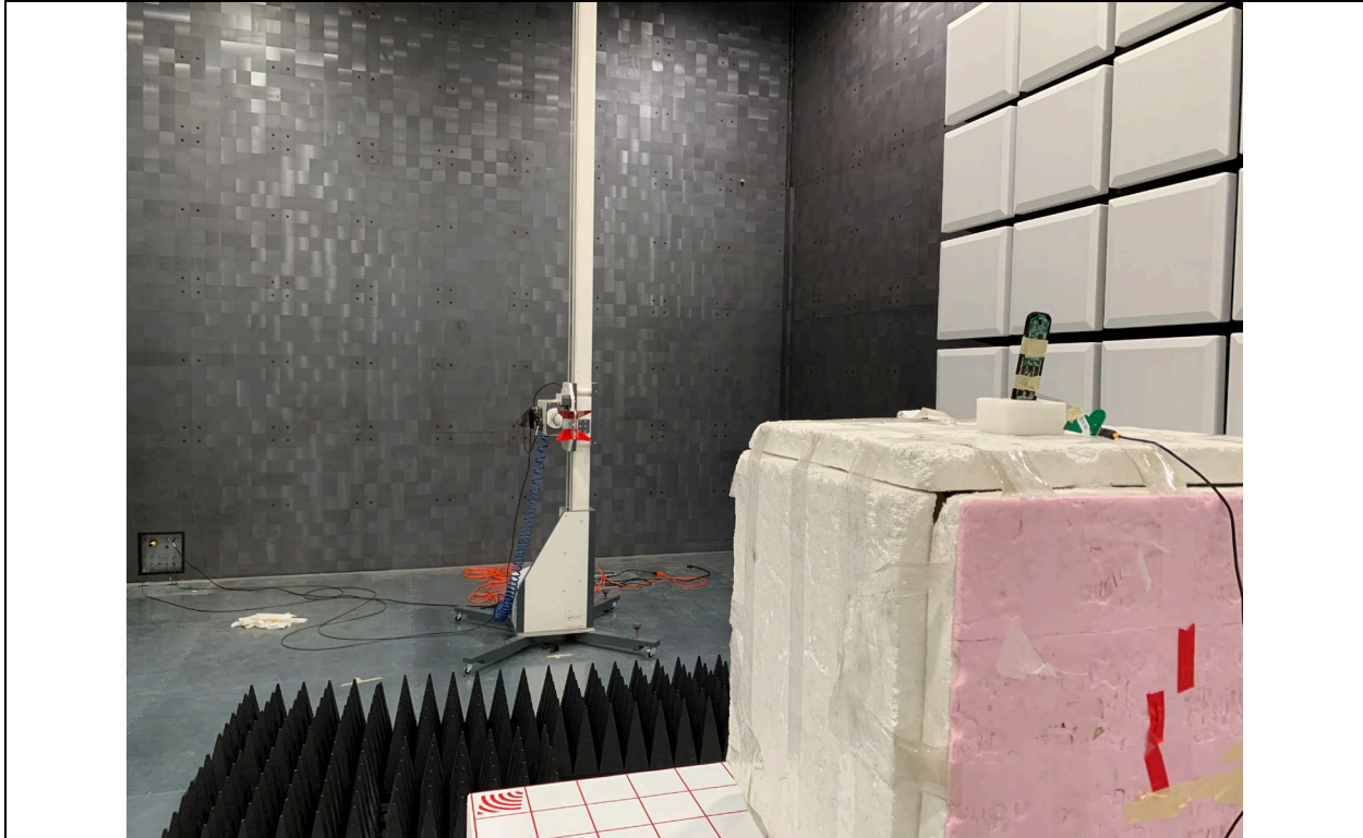
Radiated Emission Test above 1GHz Rear View
