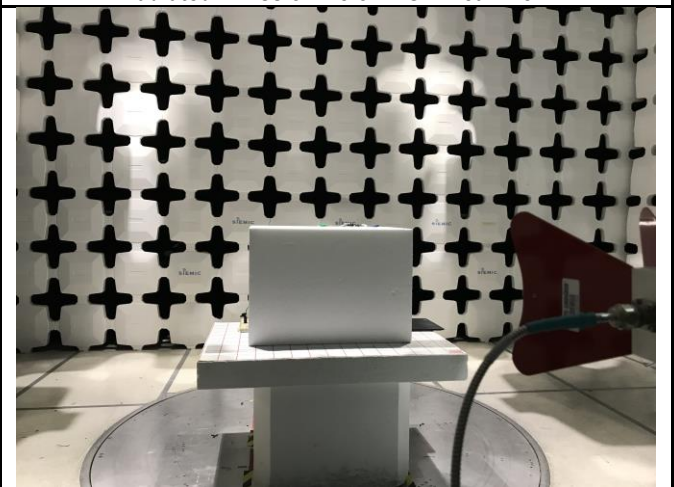
Radiated Emission Above 1G – Rear View
