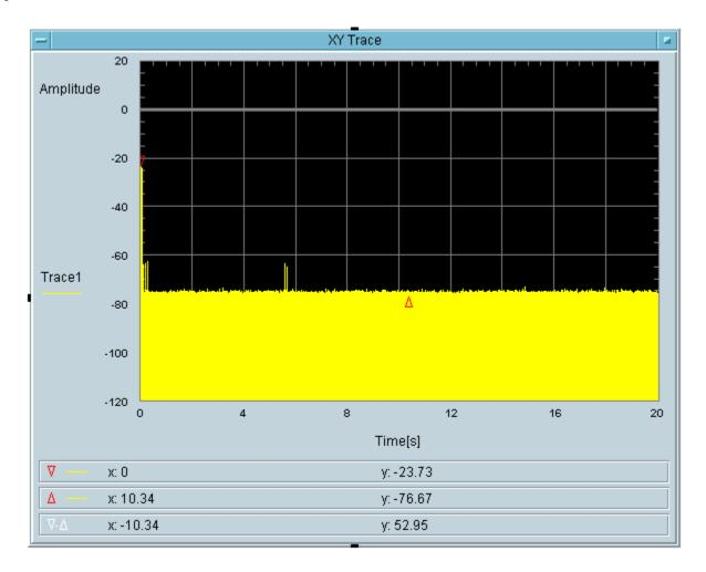
Type 0 radar channel closing transmission time result:
