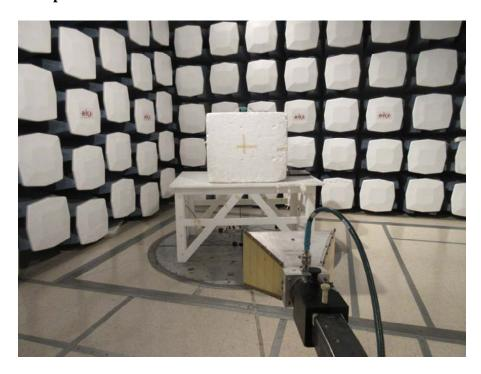
1.6 Radiated Spurious Emission above 1 GHz Rear View
