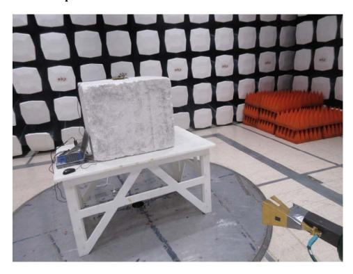
1.8 Radiated Spurious Emission 26.5-40 GHz Rear View
