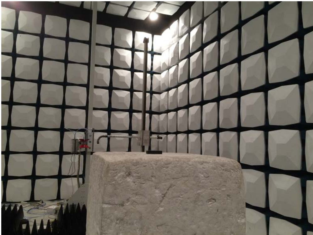
Description: Radiated Emission Test Setup for 1~18GHz
