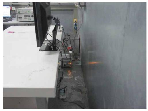
Test Mode : Transmitting Description : Radiated Emission Test Setup for Below 30MHz
