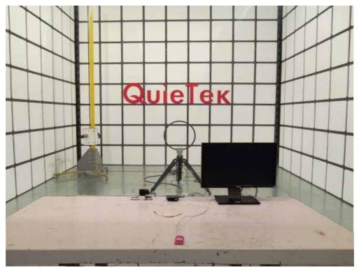
Test Mode : Transmitting Description : Radiated Emission Test Setup for Below 1GHz
