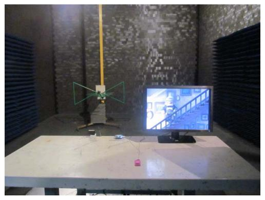
Test Mode : Transmitting Description : Radiated Emission Test Setup for 1~18GHz
