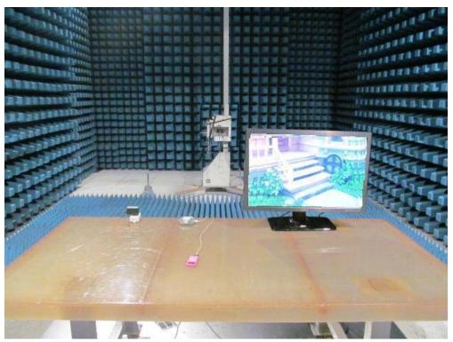
Test Mode : Transmitting Description : Radiated Emission Test Setup for Above 18GHz
