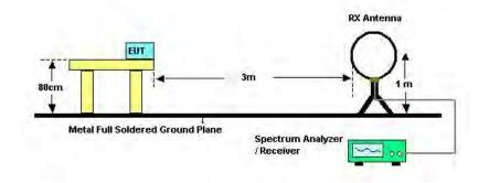
For Radiated Emissions: 30MHz~1GHz
