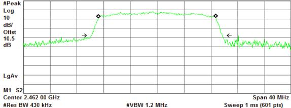
Occupied Bandwidth 17.5804 MHz Occ BW % Pwr 99.00 % x dB -26.00 dB
