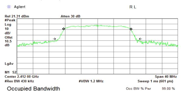
Transmit Freq Error -19.653 kHz x dB Bandwidth 19.365 MHz
