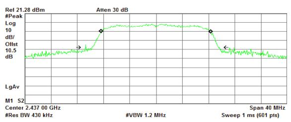
Occupied Bandwidth 16.7471 MHz Occ BW % Pwr 99.00 % x dB -26.00 dB
