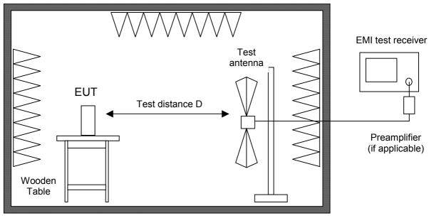
Alternate test site (semi anechoic room)
