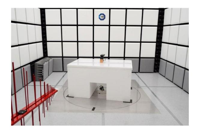
Radiated Emissions Test Setup (30 MHz to 1 GHz Front)
