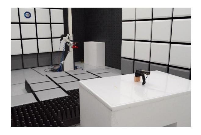
Radiated Emissions Test Setup (above 1 GHz Back)
