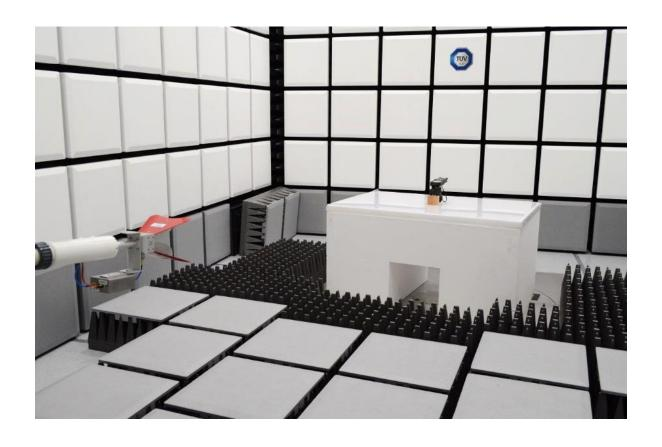
Radiated Emissions Test Setup (above 1 GHz Front)
