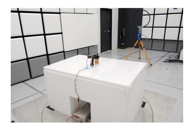
Radiated Emissions Test Setup (9 kHz to 30 MHz Back)
