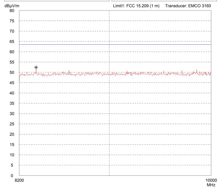
Model: MC 9090 RFID UHF Internal Antenna Serial no.: Applicant: **BARTEC GmbH** Test site: Fully anechoic room, cabin no. 2 Tested on: Test distance 1 meter Vertical Polarization Date of test: Operator: 07/29/2009 M. Steindl Test performed: File name: automatically default.emi Detector:
