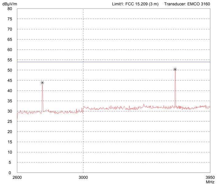
Model: MC 9090 RFID UHF Internal Antenna Serial no.: Applicant: **BARTEC GmbH** Test site: Fully anechoic room, cabin no. 2 Tested on: Test distance 3 metres Horizontal Polarization Date of test: Operator: 07/29/2009 M. Steindl Test performed: File name: automatically default.emi
