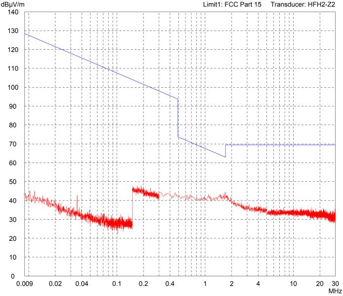
Model: MC 9090 RFID UHF Internal Antenna Serial no.: Applicant: **BARTEC GmbH** Fully anechoic room, cabin no. 2 Tested on: Test distance 3 metres Horizontal Polarization Date of test: Operator: 07/29/2009 M. Steindl File name: Test performed: automatically default.emi
