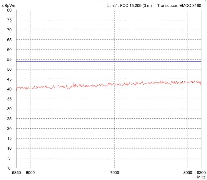
Model: MC 9090 RFID UHF Internal Antenna Serial no.: Applicant: **BARTEC GmbH** Fully anechoic room, cabin no. 2 Tested on: Test distance 3 metres Vertical Polarization Date of test: Operator: 07/29/2009 M. Steindl Test performed: File name: automatically default.emi Detector:
