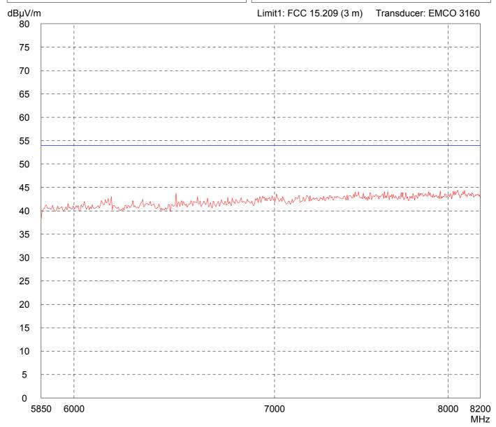
Model: MC 9090 RFID UHF Internal Antenna Serial no.: Applicant: **BARTEC GmbH** Fully anechoic room, cabin no. 2 Tested on: Test distance 1 meter Horizontal Polarization Date of test: Operator: 07/29/2009 M. Steindl Test performed: File name: automatically default.emi Detector:
