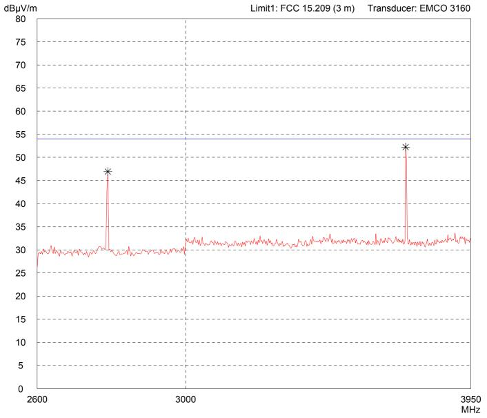
Model: MC 9090 RFID UHF Internal Antenna Serial no.: Applicant: **BARTEC GmbH** Test site: Fully anechoic room, cabin no. 2 Tested on: Test distance 3 meters Vertical Polarization Date of test: Operator: 07/29/2009 M. Steindl Test performed: File name: automatically default.emi
