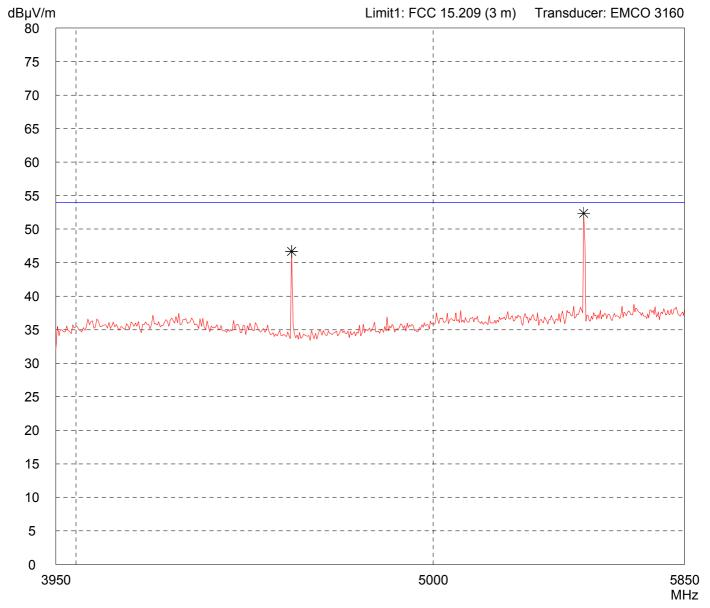
Model: MC 9090 RFID UHF Internal Antenna Serial no.: Applicant: **BARTEC GmbH** Test site: Fully anechoic room, cabin no. 2 Tested on: Test distance 3 metres Vertical Polarization Date of test: Operator: 07/29/2009 M. Steindl Test performed: File name: automatically default.emi
