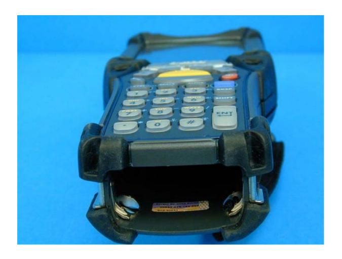
Bottom with Battery removed View
