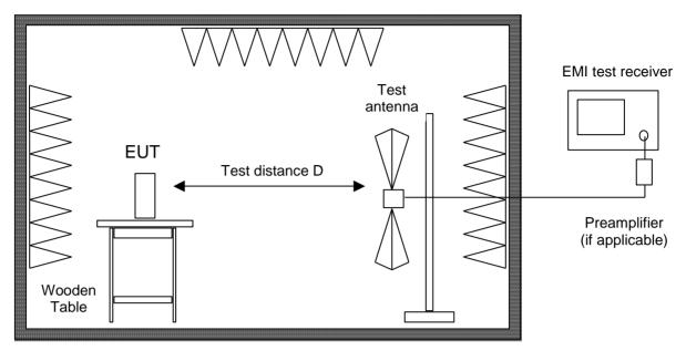
Alternate test site (semi anechoic room)
