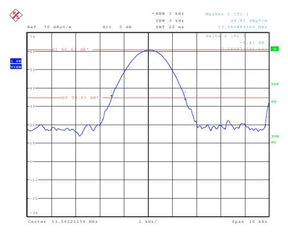
Occupied Bandwidth (-26 dB): 3.045 kHz
