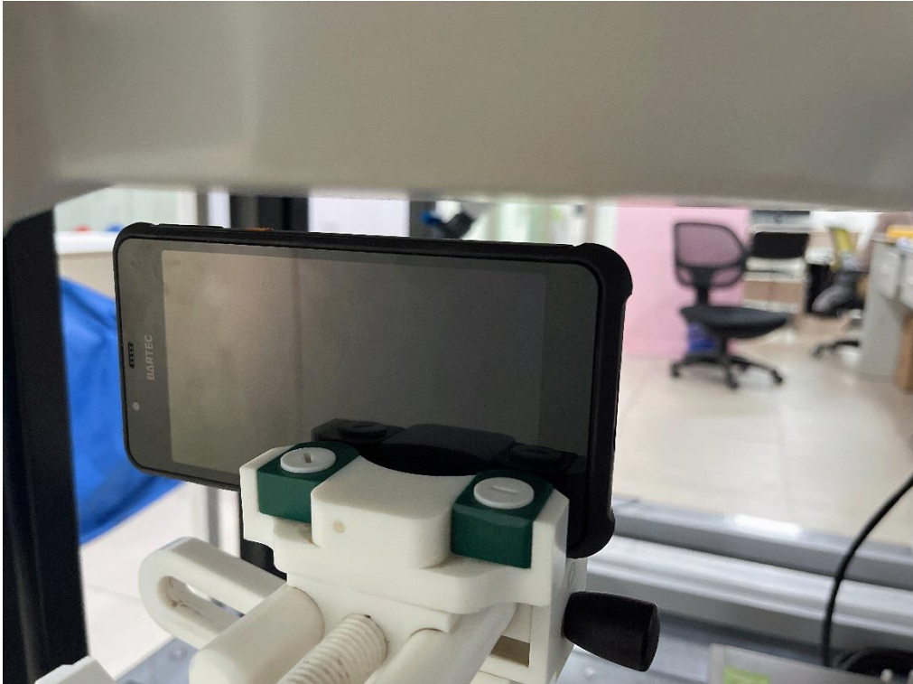
Body Right side(separation distance is 10mm)
