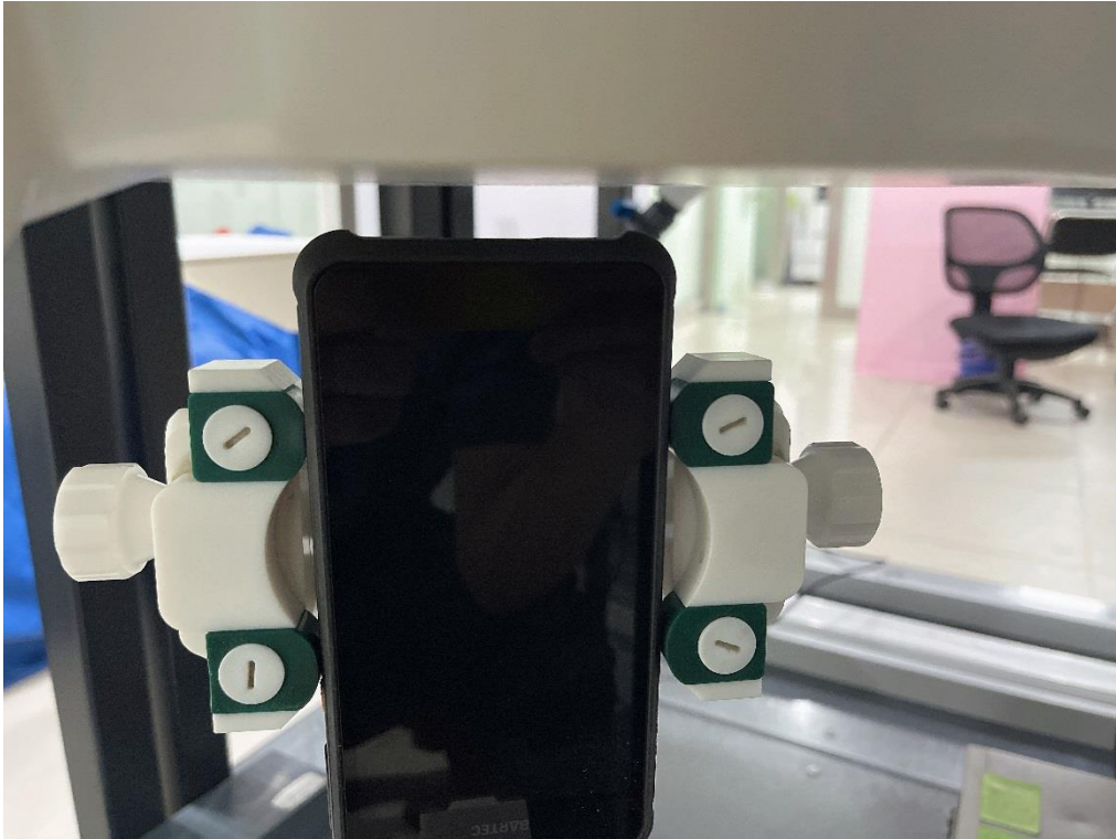
Body Bottom side(separation distance is 10mm)
