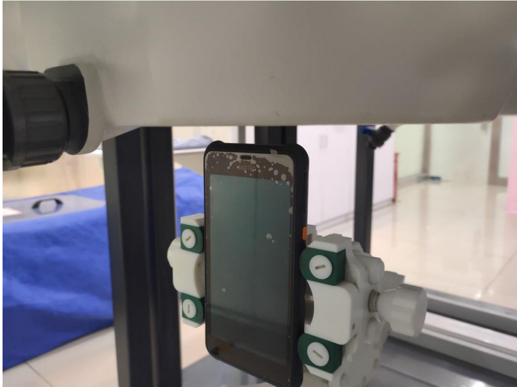
Body Top side(separation distance is 10mm)
