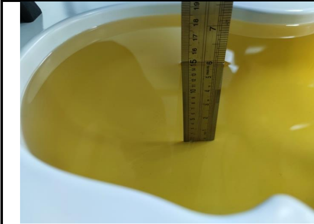
Fig. 9.1 Photo of Liquid Height for Head SAR (depth>15cm)
