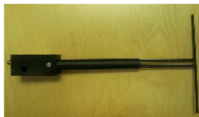
Figure 1 – MVG COMOSAR Validation Dipole
