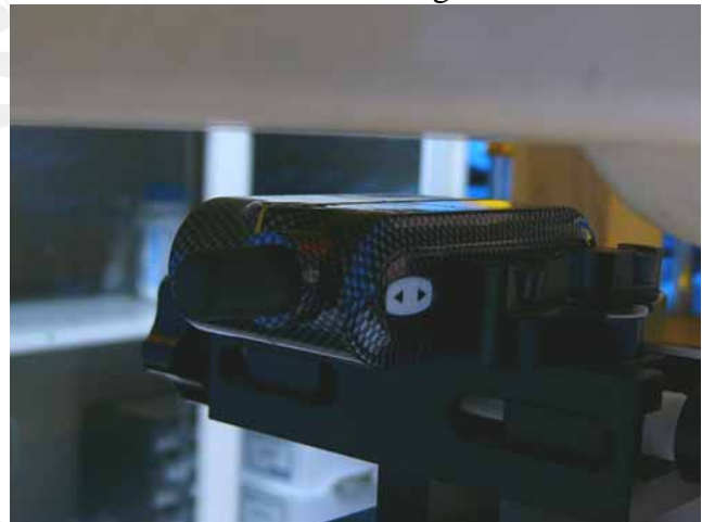
Fig.8 Body worn (EUT front to flat phantom); Testing body-worn position by separating 1.5cm between the front of the EUT and the flat phantom.
