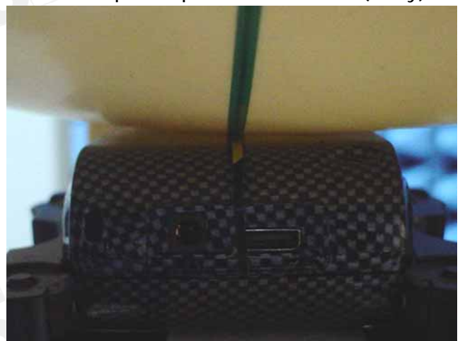
Fig.2.4 Photograph of the Tissue Simulant Fluid liquid depth 15cm for Flat (Body)
