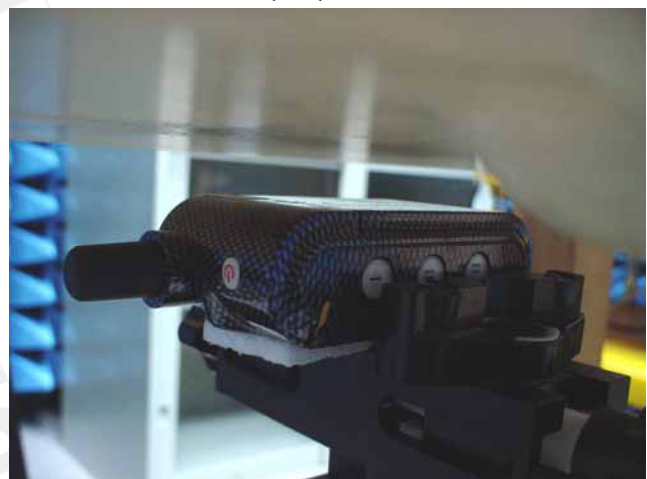
Fig.7 Body worn (EUT back to flat phantom); Testing body-worn position by separating 1.5cm between the back of the EUT and the flat phantom.
