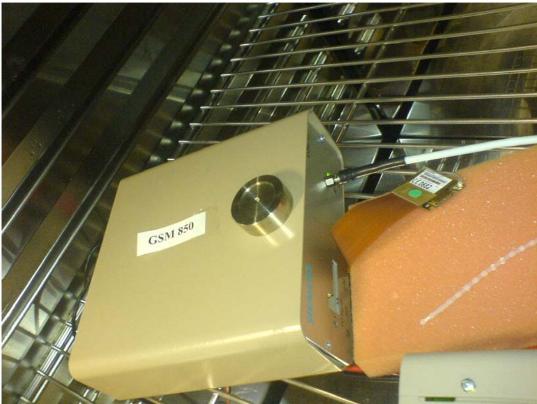
Photograph 7: Measurements in the climatic chamber, frequency stability
