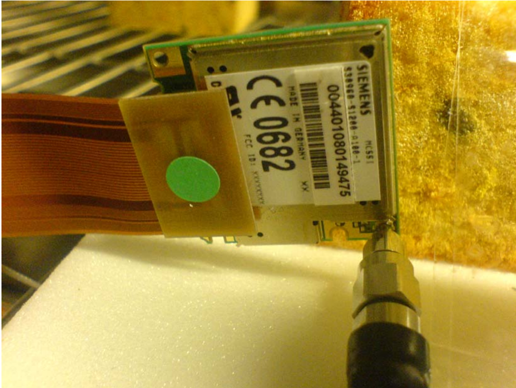
Photograph 8: Measurements of conducted power and spurious emissions on module's RF-port
