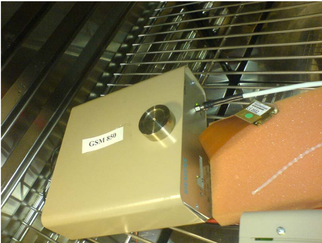
Photograph 3: Measurements in the climatic chamber, frequency stability
