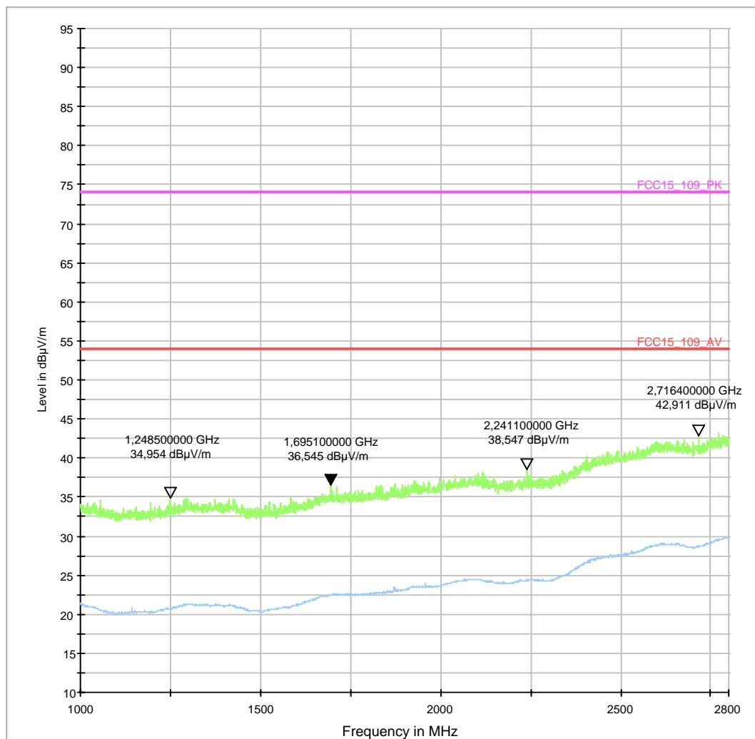
EMI Auto Test Template: 03\_1\_2.7\_ohne switch H&V
