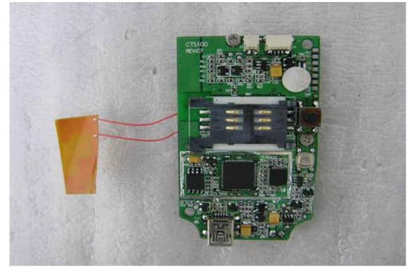
Internal View of EUT – 3 (GSM Module)
