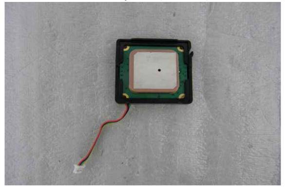
Internal View of EUT – 7 (GPS Antenna)
