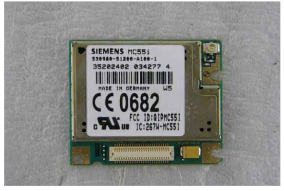
Internal View of EUT – 5 (GSM Module)
