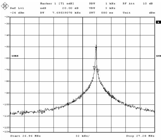
20dB bandwidth lower frequency: 27.14152MHz 20dB bandwidth upper frequency: 27.14921MHz
