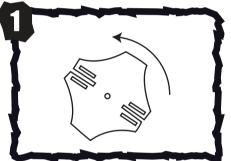
Remove the remote by turning counter clockwise the plastic keylock.
