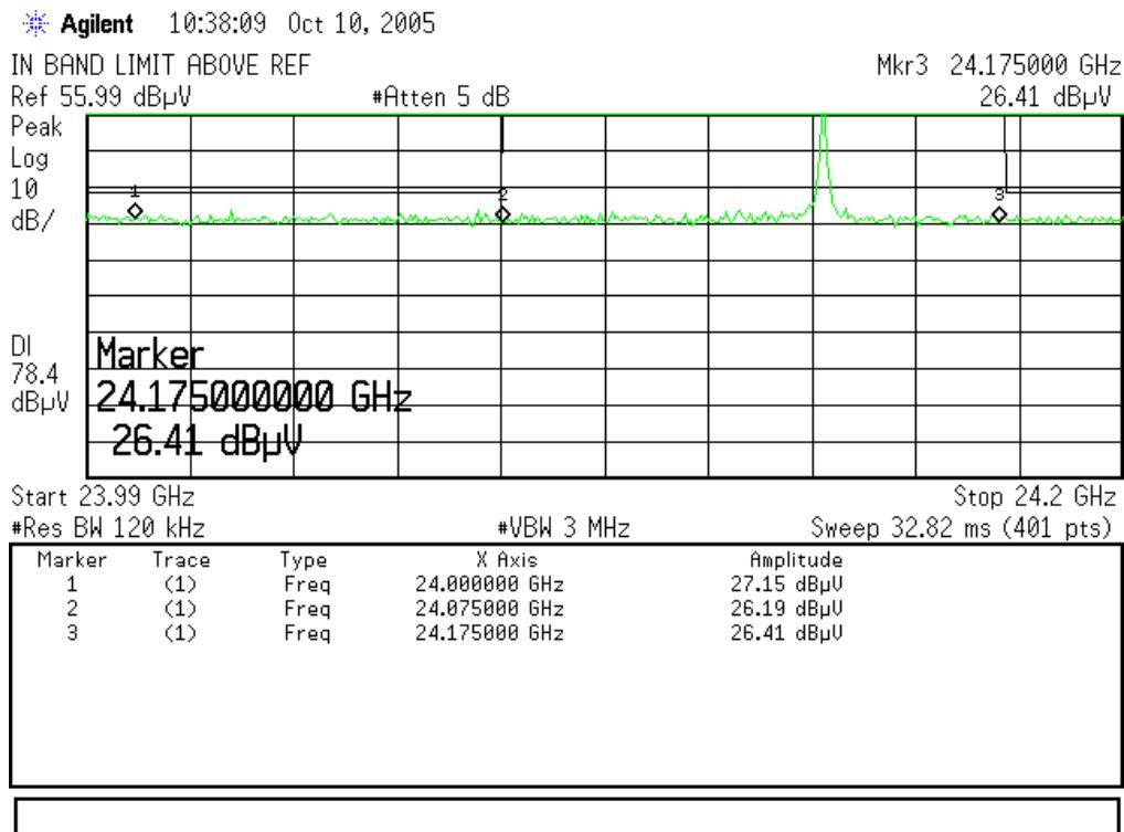
Conclusion: As seen on the above plot, the fundamental complies with the spurious limit at the bandedge.
