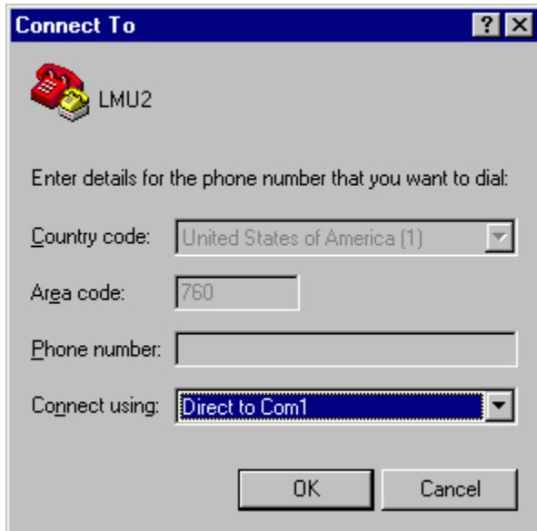
Change *Connect using* to read **Direct to ComX**. Where X is the Com port that the LMU-4000 is attached to. This will probably be Com1.
