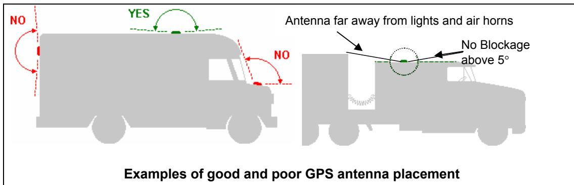
The received signal levels at the GPS antenna from the satellites are very low in power (approximately -136 dBm), so any blockage of the antenna can affect the quality of the location computed by the receiver. Kinks or tight knots in the antenna cable can also prevent the GPS receiver from operating properly. When laying out the antenna cable, care should be taken so that the cable is not subjected to crushing or strain.
