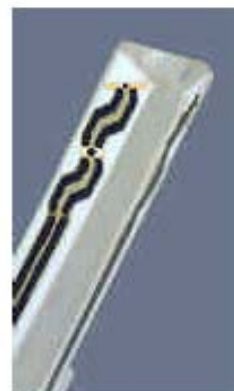
Figure 3.4 Probe Thick-Film Technique
