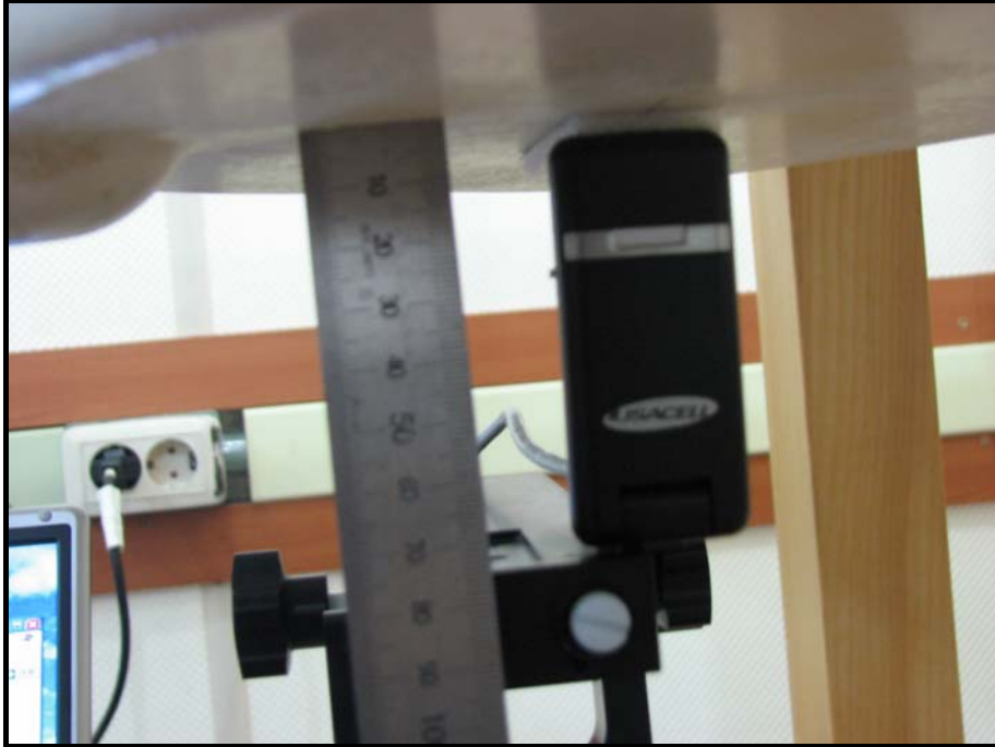
Vertical Top : The front Top side of EUT face to the Phantom with 5mm separation distance.
