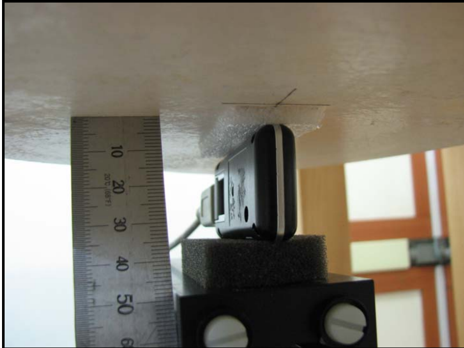
Vertical Right : The right edge of EUT face to the Phantom with 5mm separation distance.
