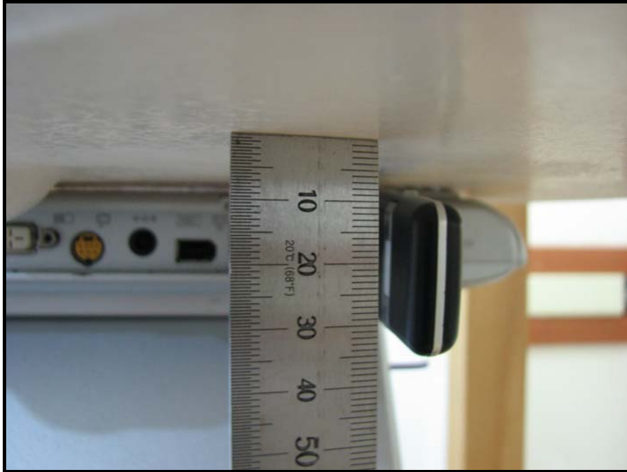
Laptop(Vertical) : The right edge of EUT face to the Phantom with 7mm separation distance.
