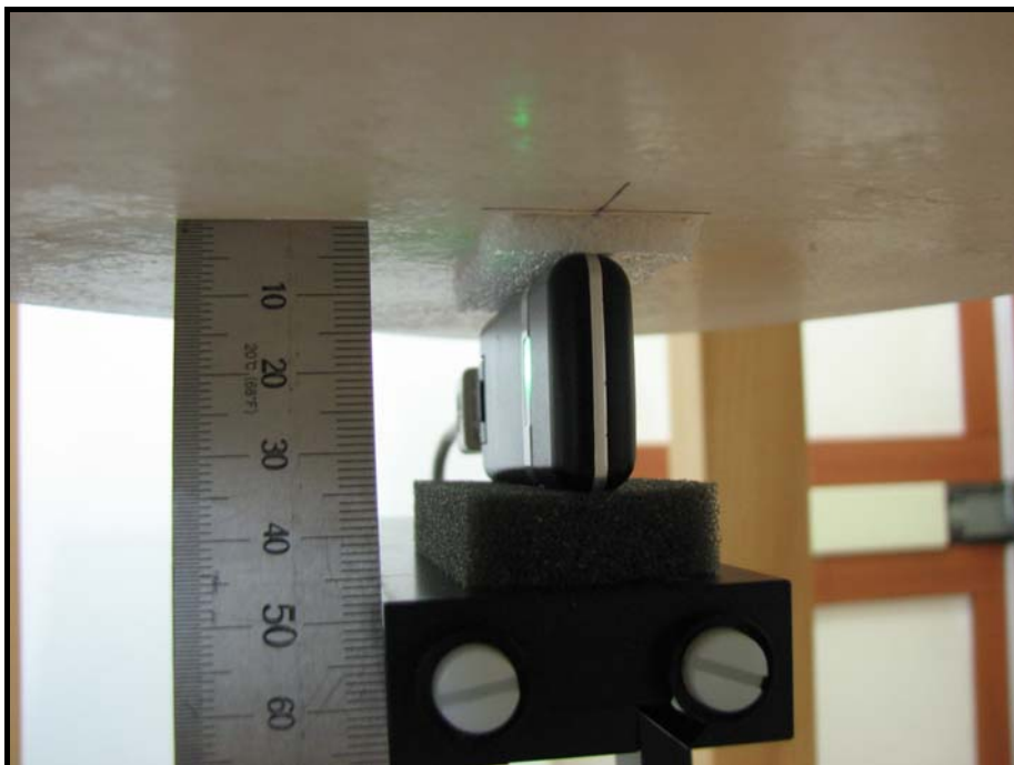
Vertical Left : The left edge of EUT face to the Phantom with 5mm separation distance.
