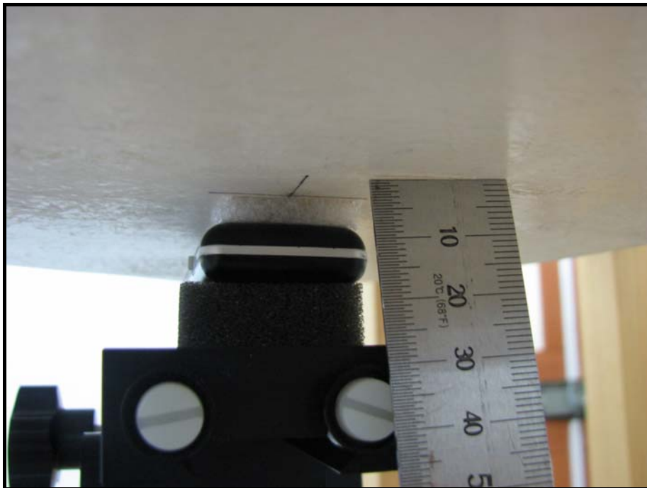
Horizontal Bottom : The bottom of EUT face to the Phantom with 5mm separation distance.
