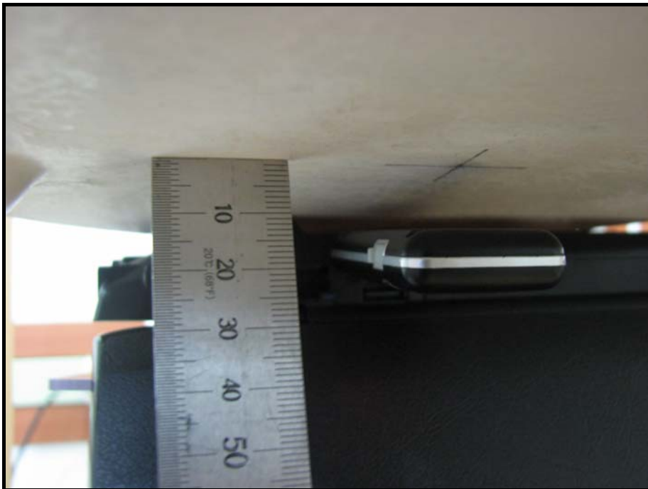
Laptop(Horizontal) : The front of EUT face to the Phantom with 10mm separation distance.
