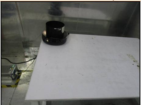
RADIATED DISTURBANCE (MAGNETIC FIELD STRENGTH) (9KHz-30MHz) TEST SETUP
