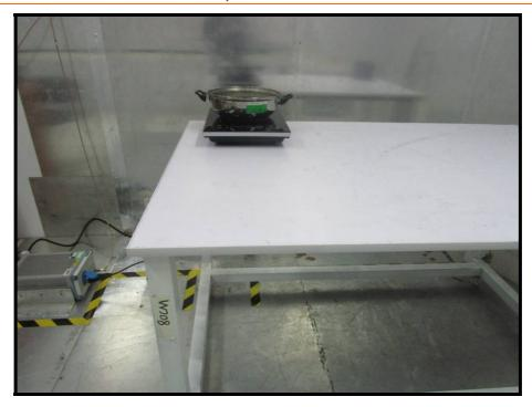
1.2 RADIATED EMISSIONS, 9 KHZ TO 30 MHZ TEST SETUP
