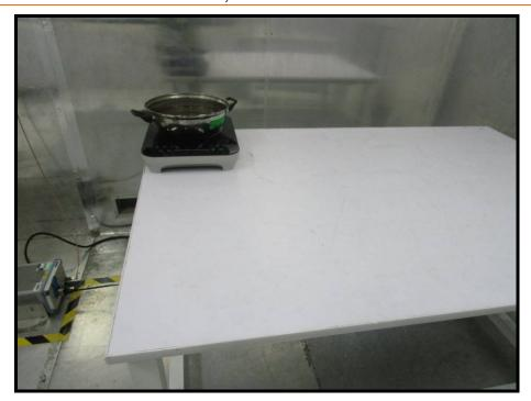
1.2 RADIATED EMISSIONS, 9 KHZ TO 30 MHZ TEST SETUP
