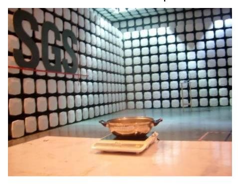
**Conducted Emissions Test Setup**
