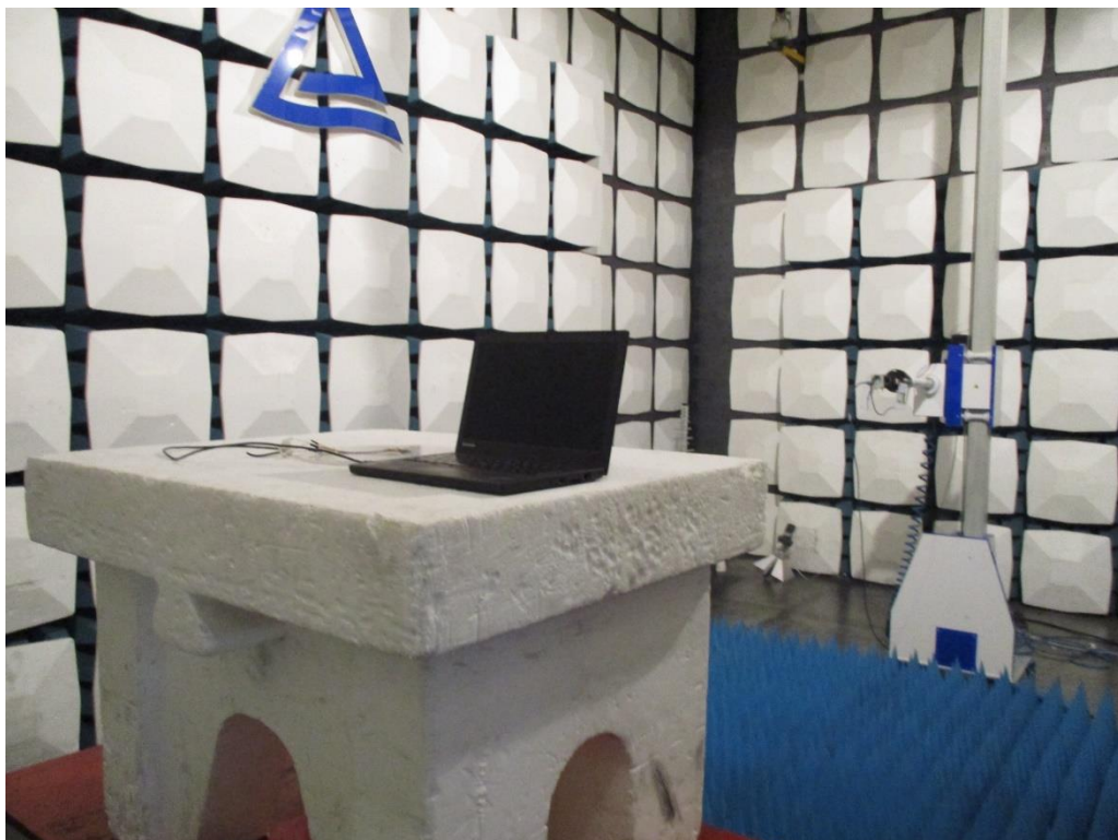
Photograph 4: Set-up for Radiated Spurious Emission, 18GHz - 26.5GHz
