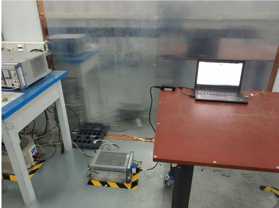
Photograph 5: Set-up for Conducted Emission on AC Mains
