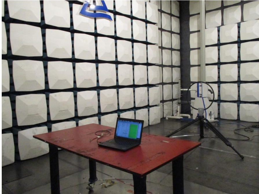
Photograph 1: Set-up for Radiated Spurious Emission, 9kHz - 30MHz
