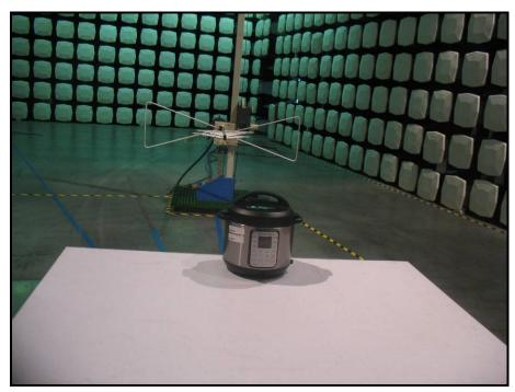
Above 1GHz: (full anechoic chamber)
