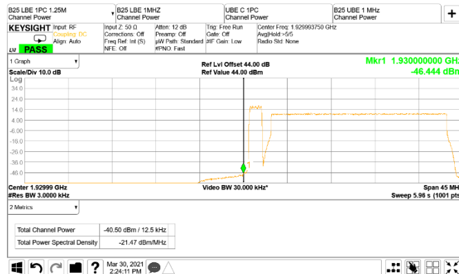
Figure 8.3-115: Conducted band edge emission at 1930 MHz, CDMA and LTE 20 MHz, antenna port B two-carrier operation (RBW = 1% of EBW)
