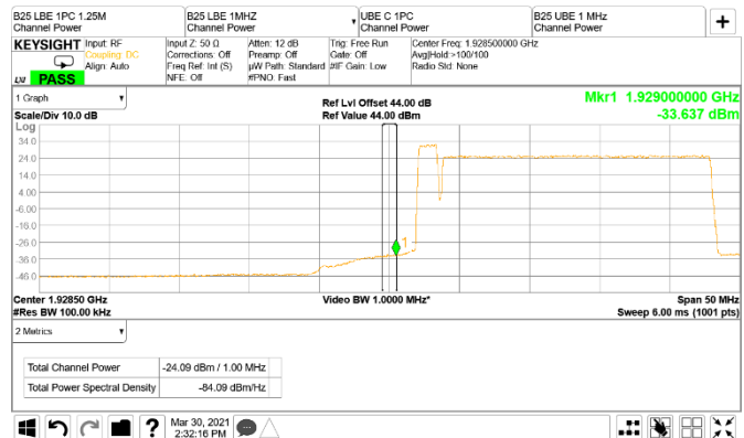
Figure 8.3-144: Conducted band edge emission at 1929 MHz, CDMA and NR 20 MHz, antenna port A two-carrier operation (RBW = 1 MHz)
