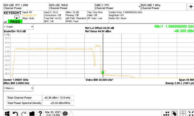
Figure 8.3-145: Conducted band edge emission at 1990 MHz, CDMA and NR 20 MHz, antenna port A two-carrier operation (RBW = 1% of EBW)
