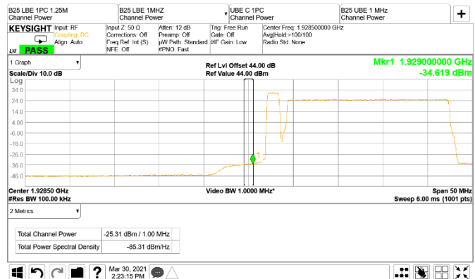
Figure 8.3-116: Conducted band edge emission at 1929 MHz, CDMA and LTE 20 MHz, antenna port B two-carrier operation (RBW = 1 MHz)
