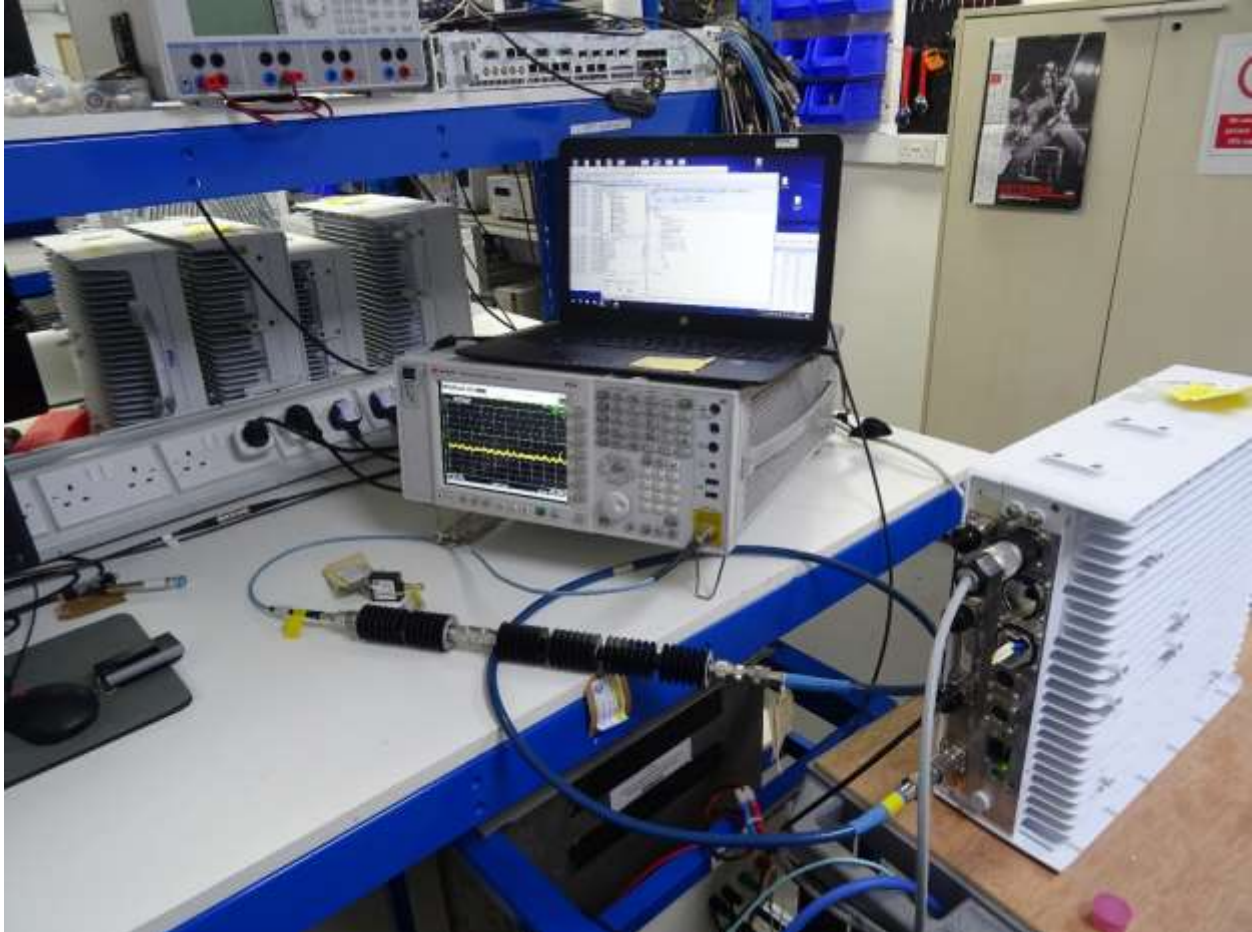
Conducted Lab Testing
