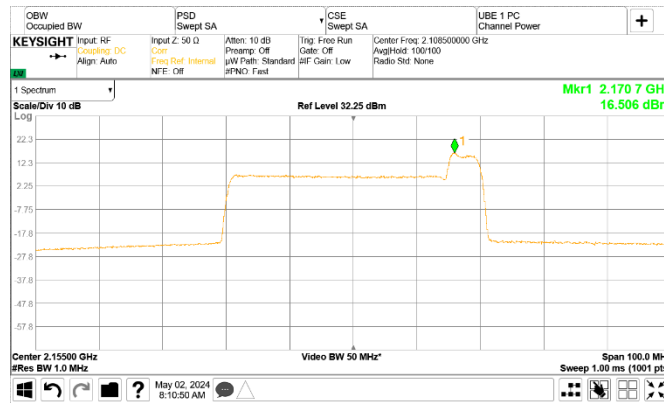
Figure 8.1-3: PSD of multi-RAT operation, NR 35 MHz + LTE with IoT1 5 MHz, Sample plot, Contiguous
