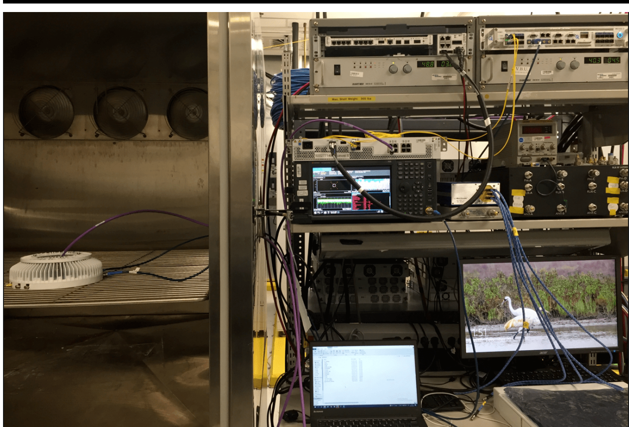
Figure 5: Conducted test setup (Frequency Stability)
