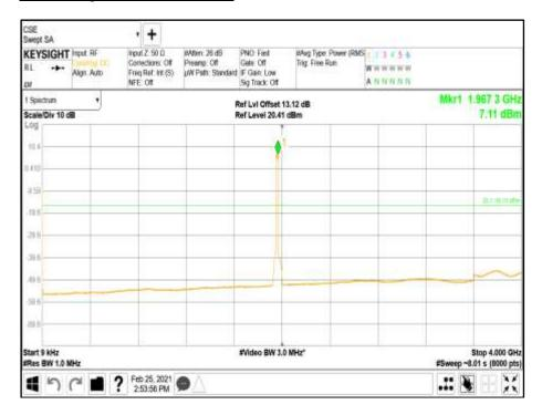
$\underline{\text{Modulation NR: QPSK - Carrier Bandwidth 5.0+5.0+5.0+5.0 MHz - Channel Position M - Band } \underline{\text{2.00 - Range 4000 to 12000 MHz}}$
