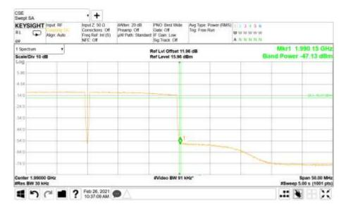
Modulation NR: QPSK - Carrier Bandwidth NR: 20.0 +20.0 MHz - Channel Position B
