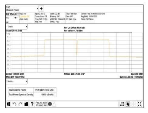
Antenna A - Modulation NR: QPSK - Carrier Bandwidth 20.0+20.0 MHz - Channel Position M
