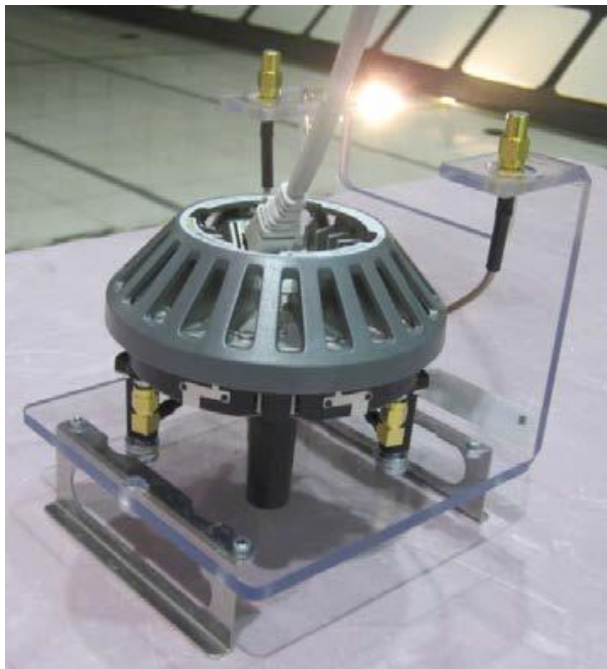
Figure 2: The EUT, RD 2242 B4 (With Test fixture)
