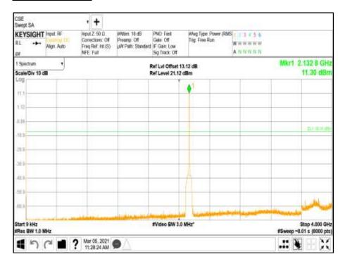
Modulation NR: QPSK - Carrier Bandwidth 5.0 MHz - Channel Position M - Band 2 - Range 4000 to 12000 MHz
