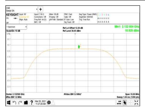
Antenna Port A Carrier Power - Modulation NR: QPSK - Carrier Bandwidth 10.0 MHz - Channel Position M
