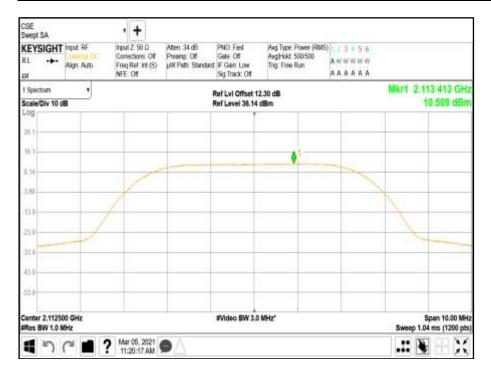
Antenna Port A Carrier Power - Modulation NR: QPSK - Carrier Bandwidth 10.0 MHz - Channel Position B
