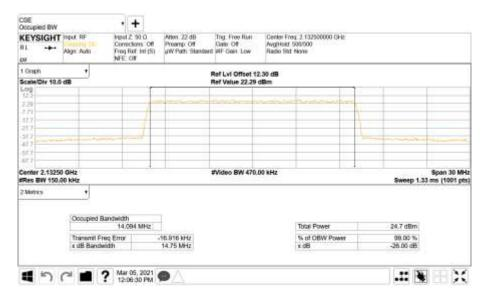
Antenna A - NR Modulation QPSK - NR Carrier Bandwidth 20.0 MHz 15 kHz SCS - Channel Position M
