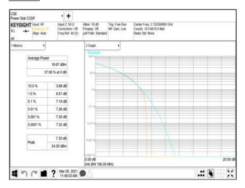
Antenna Port A PSD - Modulation NR: QPSK - Carrier Bandwidth 10.0 MHz - Channel Position M
