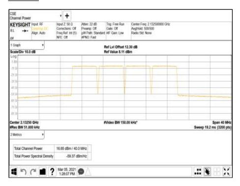
Antenna A - Modulation NR: QPSK - Carrier Bandwidth 10.0+10.0+10.0+10.0 MHz - Channel Position M
