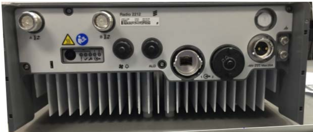
Figure 6: Radio 2212 B66A Bottom / Connector View
